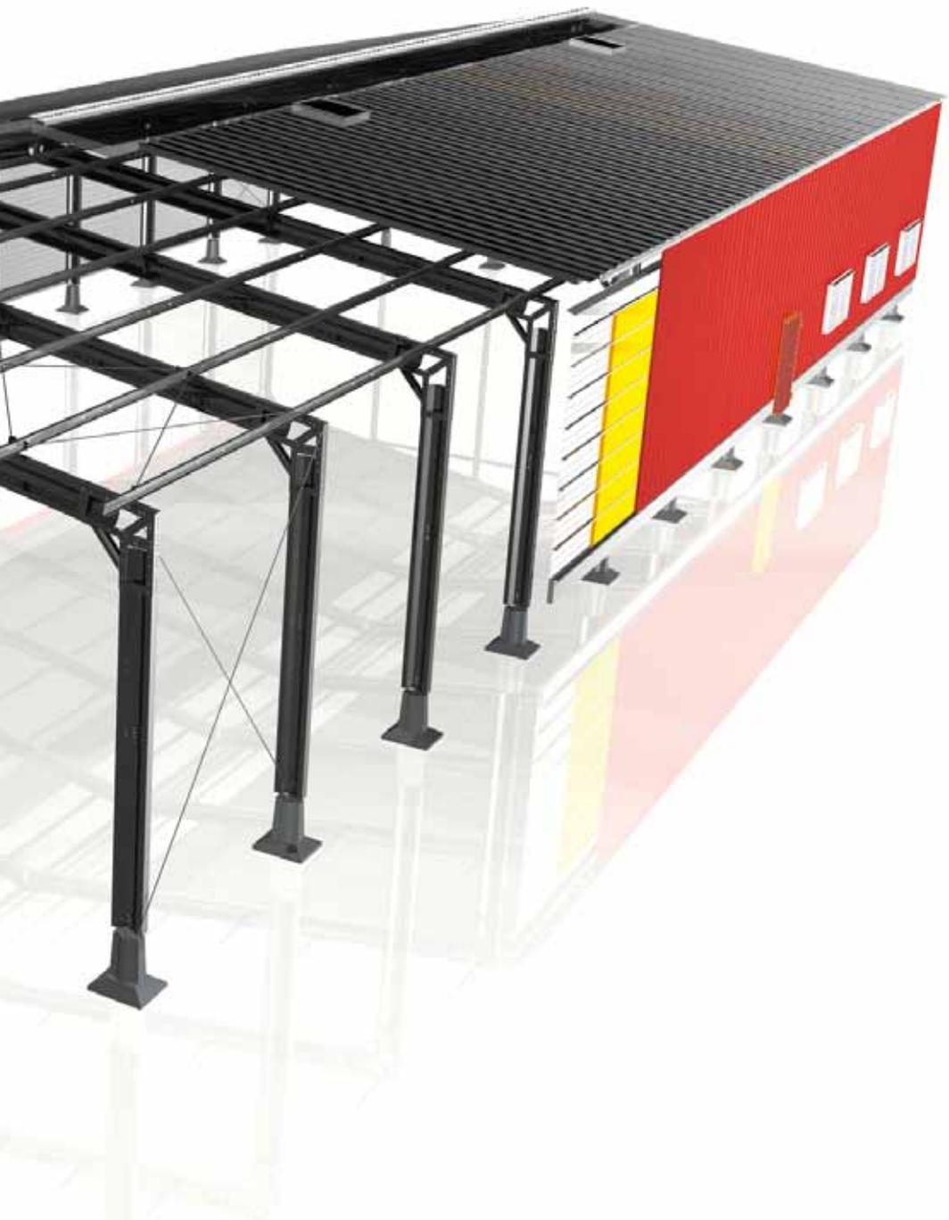
Depending on site circumstances and local regulations, Astrigma buildings can be installed on prefabricated concrete elements or purpose-built foundations. The adapted anchor sets or expansion bolts secure the building to **resist the strongest forces.**
